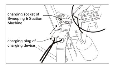
The charging process lasts for approx. 10 hours when the batteries have been completely used up (with the device originally provided by the manufacturer).
