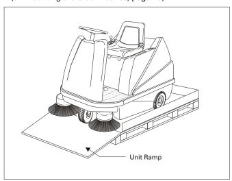
Drive the Sweeping & Suction Machine over a ramp out of the transport packaging. (Cf. page 8, Driving)
