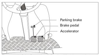
The speed of the Sweeping & Suction Machine can be adjusted with infinite variability by depressing the accelerator.
