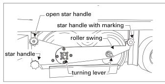
Pull the sweeping rollers out of the machine and remove any debris, cords, etc., from the roller tunnel and from the pick-up pins.
