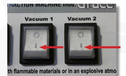
Run vacuum for 10 minutes with the top dome removed. This will dry out any moisture that is sitting near the motor.
