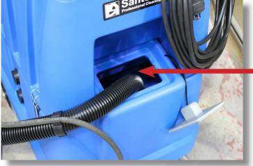
Drain solution tank if machine won't be used within the next 7 days. You can suck this into the top tank by removing the cuff from the wand.
