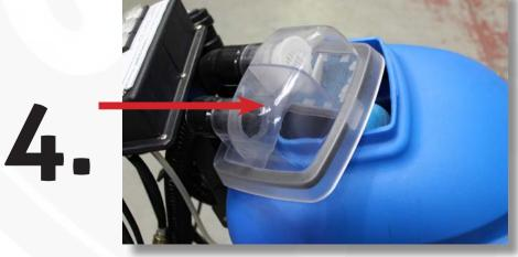
Always leave clear dome to one side or upside down. This will help the tank not to condensate, consequently extending the life of the vacuum motors. 5.
