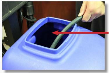
Clean out top recovery tank thoroughly, flush with clean water.
