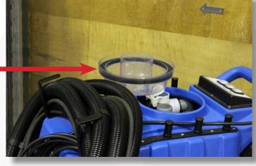
Always leave clear dome to one side or upside down. This will help the tank not to condensate, consequently extending the life of the vacuum motors.
