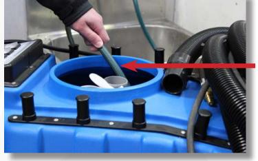
Clean out top recovery tank thoroughly, flush with clean water.
