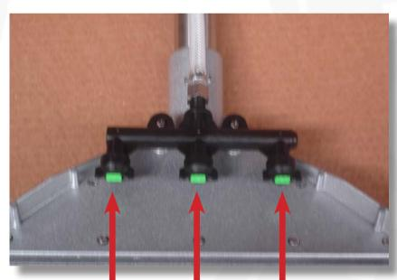
Remove jet nozzles and holders, clean out regularly. Replace nozzles when they lose their ability to evenly fan the water spray.
