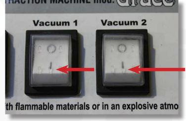
Run vacuum for 10 minutes with the top dome removed. This will dry out any moisture that is sitting near the motor.
