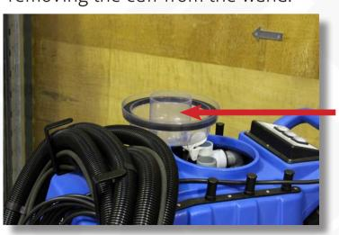
Always leave clear dome to one side or upside down. This will help the tank not to condensate, consequently extending the life of the vacuum motors.
