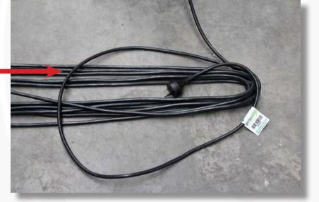
Check power lead for visual damage, do not use if damaged.
