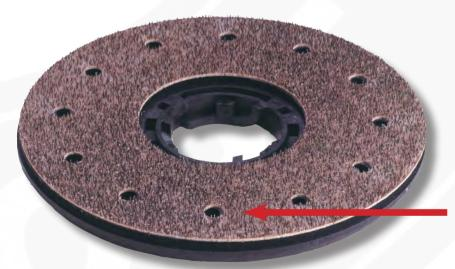
Check brush or pad drive for wear or damage. Replace as necessary.
