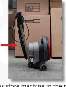
Always store machine in the position shown. This will prevent damage to the brush/pad drive.
