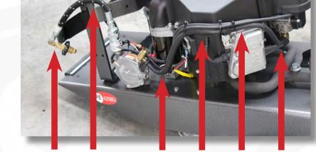
Inspect gas connections for damage or abrasions. Get damaged parts replaced by your technician.
