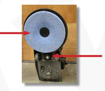
Inspect Pad & Belts for wear/damage, refer to manual for details.
