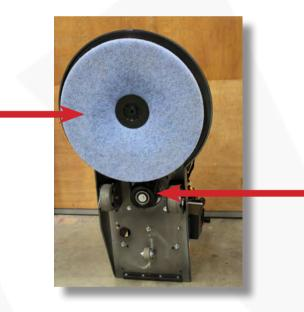
Remove Pad and inspect Pad & Belts for wear/damage, refer to manual for details.
