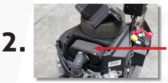
Check Air Filter for debris. (Undo the 2 plastic knobs to remove the Filter cover).
