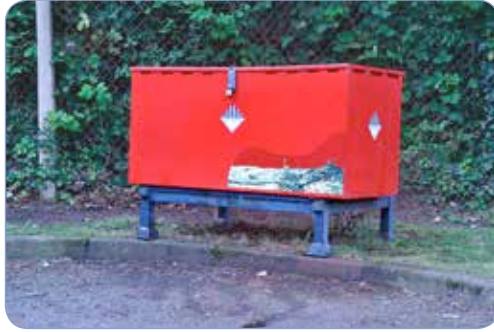
An example of a waste battery storage bin well away from buildings.
