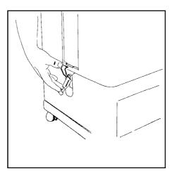
2. Fill the solution tank with cold or warm water, through the filling hole, adding a 5% of nonfoaming detergent (1/2 liter in 10 liters). Higher concentrations may be used in case of particularly dirty surfaces.
