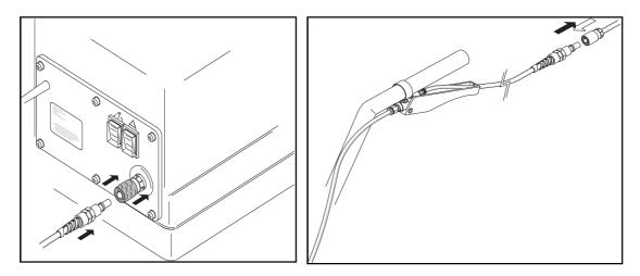
5. In the same way, you must connect the vacuum hose to the machine and to the accessory handle.
