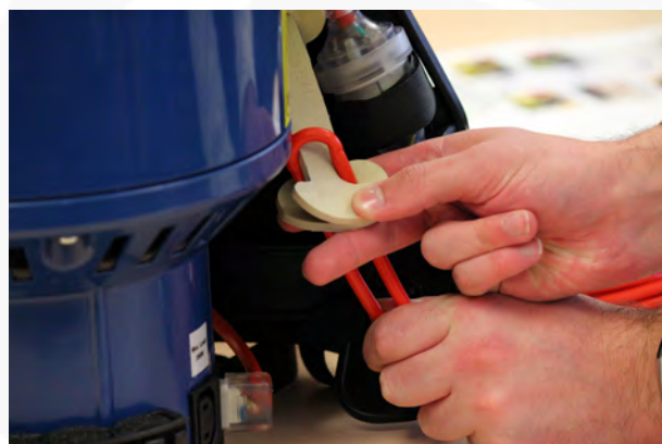
Poke cord restraint tongue through cable loop, then pull lead back through cord restraint, firmly against tongue.
