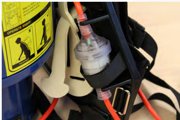
Attach orange extension lead to short lead and fasten into cradle with velcro strap.
