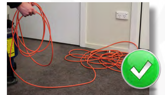
Always wind up the lead from the machine end, this helps to prevent the lead from twisting.
