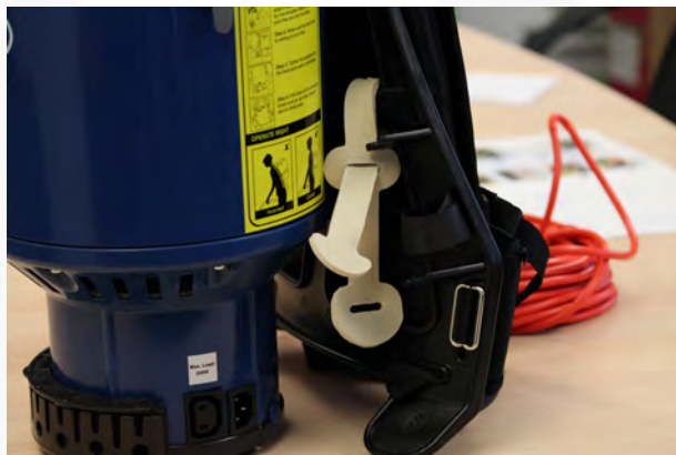
Attach and loop the white cord restraint onto the frame support.
