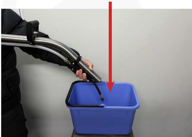
Disconnect wand from hose and turn upside down over a drain. This will empty the wand of water to keep it in good condition when not in use.
