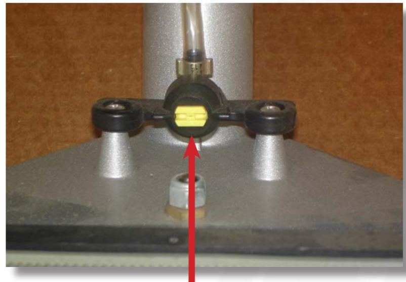
Remove jet nozzle and holder, clean out regularly. Replace nozzle when it loses its ability to evenly fan the water spray.
