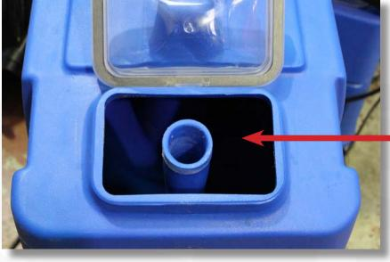
Always leave clear dome to one side or upside down. This will help the tank not to condensate, consequently extending the life of the vacuum motors.
