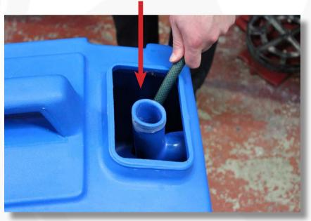
Clean out top recovery tank thoroughly, flush with clean water.
