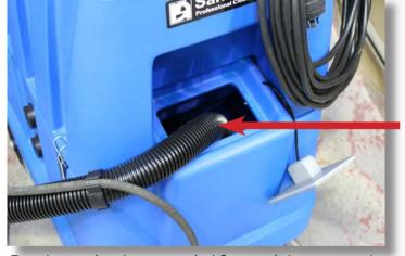
Drain solution tank if machine won't be used within the next 7 days. You can suck this into the top tank by removing the cuff from the wand.
