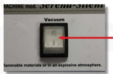
Run vacuum for 10 minutes with the top dome removed. This will dry out any moisture that is sitting near the motor.
