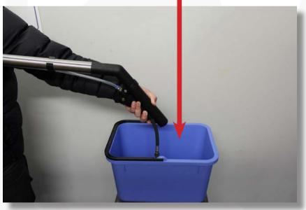
Disconnect wand from hose and turn upside down over a drain. This will empty the wand of water to keep it in good condition when not in use. 2.
