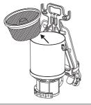
2. Remove and tap gently to clean HEPA filter (flat HEPA filter in micron 700).
