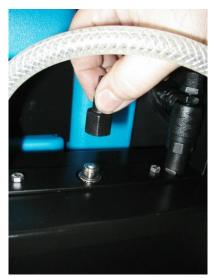
This operation allows the water to go out of the pipe, even if the pipe is not connected with any accessory.
