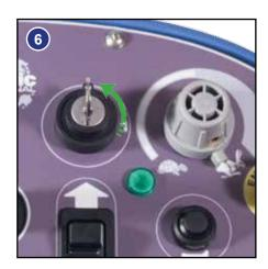
Insert key into ignition and turn quarter-turn clockwise to the 'ON' (1) position, make sure that the forward / reverse switch is set to forward and the speed control is set to low (Fig.4).
