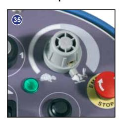
Use the maximum speed control knob and set desired traction speed as required, depending on floor type and level of soiling (Fig.35).
