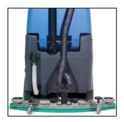
When filling the clean water tank, do not fill above the clean water tank emptying hose retaining clip (Fig.25). This can be found at the rear of the machine.
