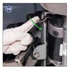
The Free-wheel lever can be found on the right hand side of the rear axle (Fig.58). To disengage the brake, pull the lever into the down position (Fig.59). Re-engage the brake by moving the lever into the up position.
