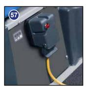
The large capacity gel batteries are sealed for life and are totally maintenance free. The on-board charger automatically monitors the charging process and will switch off when the batteries are fully charged.
