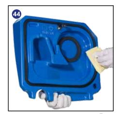
Before removing the separator, first pull off the connected hose (Fig.42). Remove the separator and rinse using clean water (Fig.43). The separator also has a sealing-rubber which should be examined at every clean-down (Fig.44).
