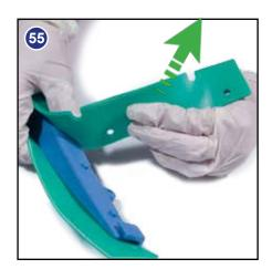
Periodically the floor-tool blades should be examined and checked for wear and damage. The blade removal is easy. Simply start by removing the four retaining pins (Fig.52), turn the floor-tool over and separate the blade carrier from the body (Fig.53-54). Peel away the blades from their locating lugs (Fig.55) and examine or renew as required. Replacement is a reversal of the removal process.
