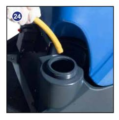
To fill the clean water tank extend the Flexifill hose, remove the rubber seal and fill from a suitable water outlet (Fig.22). Replace seal and hose to original position when finished.
