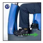
To lower the brush deck slide the brush deck foot pedal forward with your foot (Fig.14) and gently release the foot pedal (Fig.15). The brush deck is now in the lowered position.
