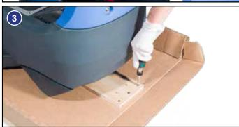
Lift top tank assembly to reveal battery compartment. Always lift between points as illustrated to ensure personal safety (Fig.1). Fit battery fuse into the battery fuse holder as illustrated (Fig.2). Remove transit block from pallet (Fig.3).
