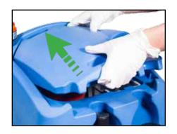
When refitting the separator make sure you engage the tab (A) at the front of the separator BEFORE pushing the separator down.
