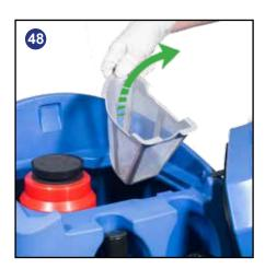
Located in your waste water (top) tank is a vacuum shut off system, this prevents suction when the waste water tank is full. It also prevents foam created by high-foaming detergents from entering the motor. Sometimes the float vents get clogged and blocked, clean to ensure correct operation (Fig.46-47) reguarlly check and clean the air filter in the top of the assembly.
