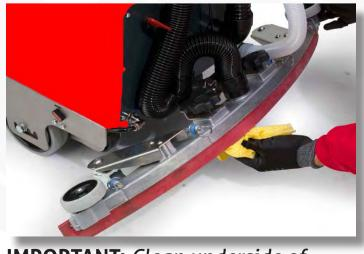
**IMPORTANT:** Clean underside of squegee from dirt and debris.
