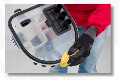
Ensure the seperator is clean and undamaged. Replace seal if necessary.
