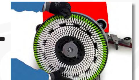
Remove brushes/pad drives and check for wear and damage.
