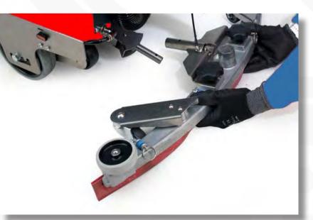
**IMPORTANT:** Remove squegee and check for wear and damage. Clean thoroughly.
