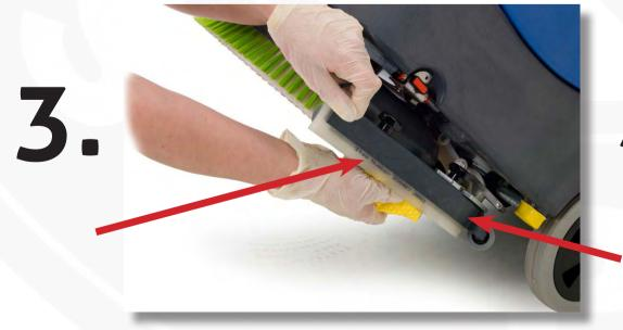
Remove squegee and check for wear and damage. Clean thoroughly.
