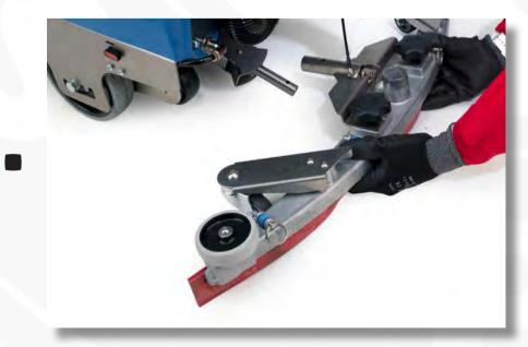
Remove squegee and check for wear and damage. Clean thoroughly.
