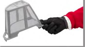
Clean out the debris filter basket located under the seperator hood.
