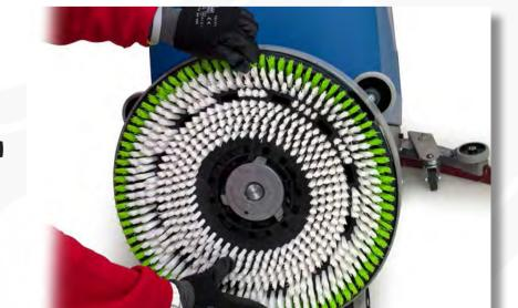
Remove brushes/pad drives and check for wear and damage.
