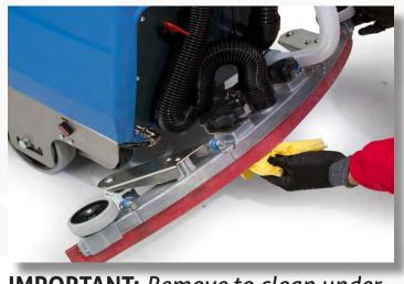
**IMPORTANT:** Remove to clean underside of squegee from dirt and debris.
