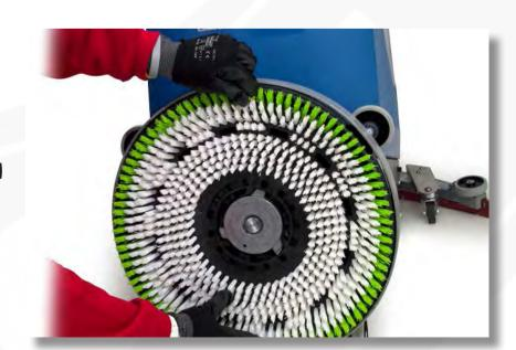
Remove brushes/pad drives and check for wear and damage.
