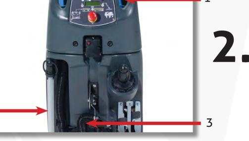
Check all hoses for damage, holes and obstructions. Clean and replace as necessary.
