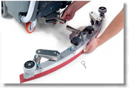
**IMPORTANT:** Remove squegee and check for wear and damage. Clean thoroughly.
