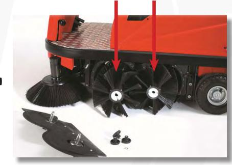
Remove the brooms and inspect for any trapped debris.
