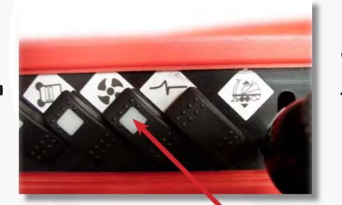
Rumble the dust filter for 15 seconds.
