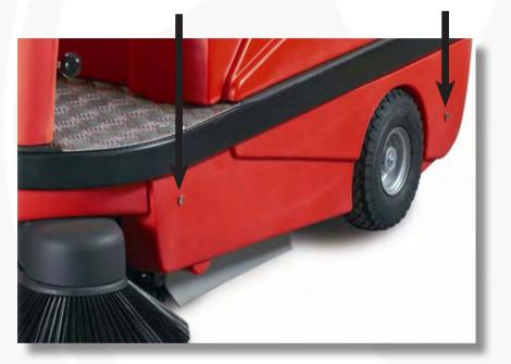
Remove the 2 screws on the left side panel.
