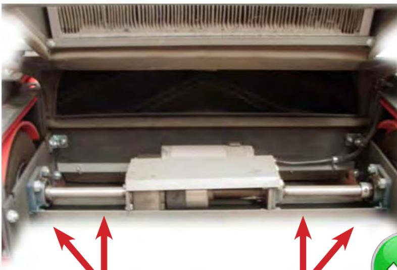
Check for and remove any trapped debris that may be caught in or around the main brooms.
