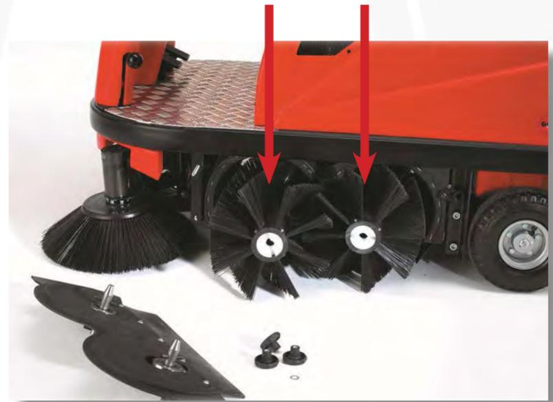
Remove the brooms and inspect for any trapped debris.
