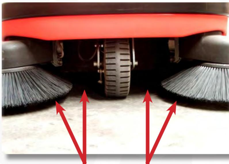
Check the front of the machine and the side brooms for any trapped debris.
