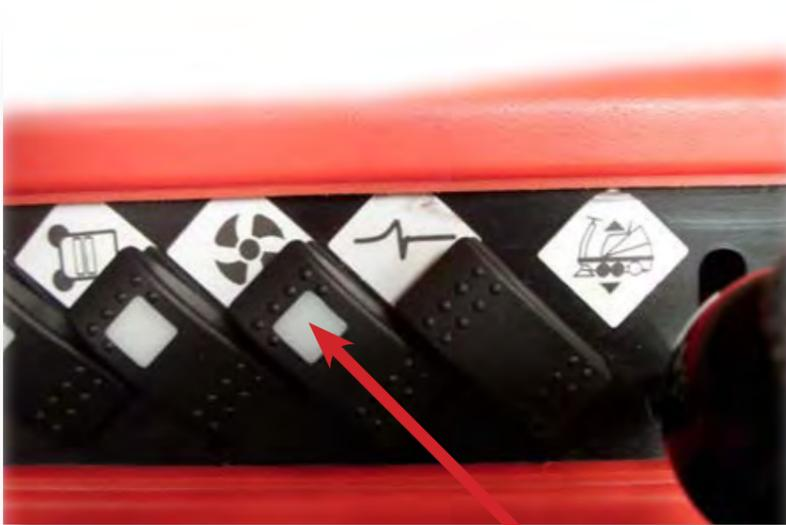
Rumble the dust filter for 15 seconds.
