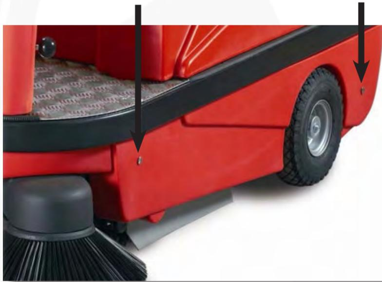
Remove the 2 screws on the left side panel.
