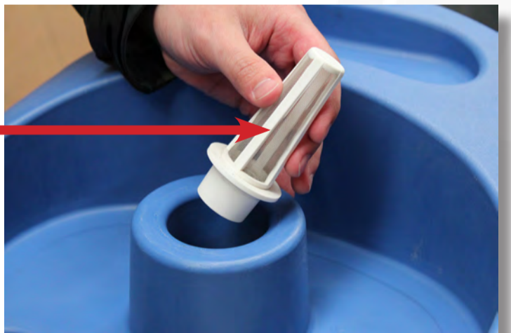
Clean suction pod filter, keep this dry.
