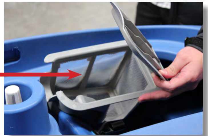
Clean out the debris filter basket.
