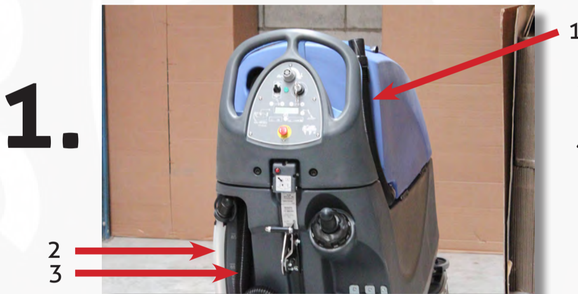
Check all 3 hoses for damage, holes and obstructions.
