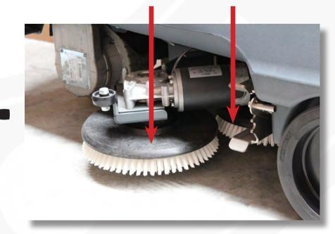
Remove brushes/pad drives and check for wear and damage.
