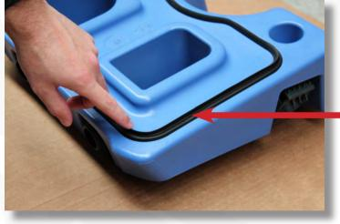
Check the seperator seal for debris or damage.
