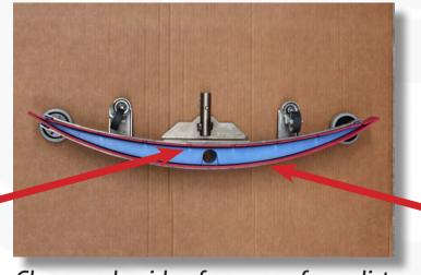
Clean underside of squegee from dirt and debris.
