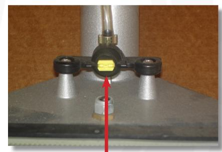
Remove jet nozzle and holder, clean out regularly. Replace nozzle when it loses its ability to evenly fan the water spray.
