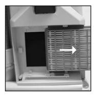
Activate the cursor N to release the ventilation grille and at the same time slide out the grille (in the direction of the arrow) to free it. The prefilter is located in the air outlet area under the Hepa filter. Replace or clean the prefilter by washing it with water, then dry it and put it carefully back in place. Refit the HEPA filter and ventilation grid, sliding it in until you hear the cursor click into place.
