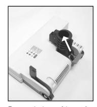
Remove the base of the appliance (see the appliance assembly chapter).
