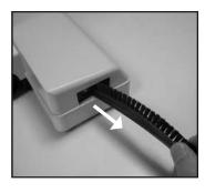
**IMPORTANT NOTE:** Before proceeding with this operation, switch off the appliance and unplug it. Use a coin or flathead screwdriver to loosen the screw fastening the cover completely Q. Use a tool (e.g. a pair of pliers), to remove the hair-covered, worn strip then replace it with another, following thesesteps in reverse order to fit it.
