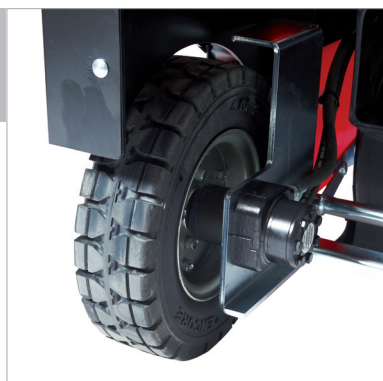
Rear-wheel drive for combustion engine versions
