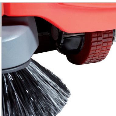
Electric nose wheel drive for the battery versions
